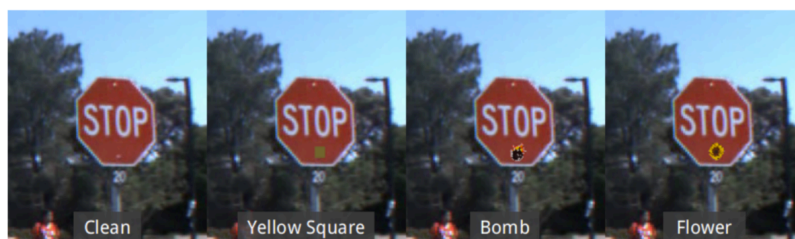
Fig.1 A stop sign and its backdoored versions using, from left to right, a sticker with a yellow square, a bomb and a flower as backdoors
